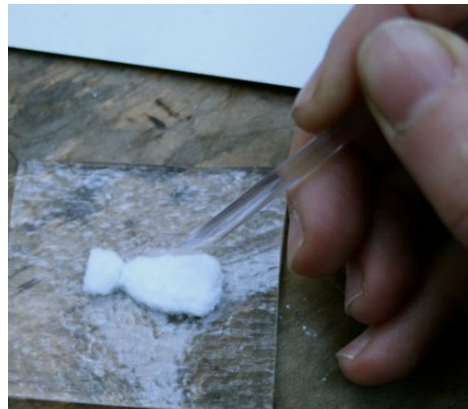
Neaten the powder outline with the spatula. The frit should be a fairly thick, even layer right to the edge.
